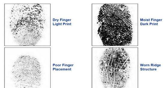
Figure 1: poor image quality: dry/wet finger, alignment and worn ridge structure (Source NIST)
