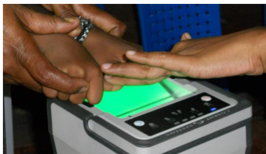
Figure 2: How to use a contact based fingerprint scanner
